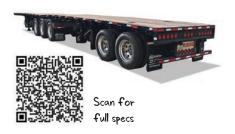
8'.6" wide x 32' & 28' Decks, Tube Side Rail, 11R-22.5 Tires, Aluminum Wheels, Load Winches, Tarp Hooks, Load sensing lift assemblies on 1st, 2nd, and 4th axles, (4) Storage Boxes, Mudflap Package, Multiple in stock
