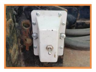
Hydraulics for the system are self-contained and require minimal maintenance. Easily raise and lower the tower with a toggle switch.
