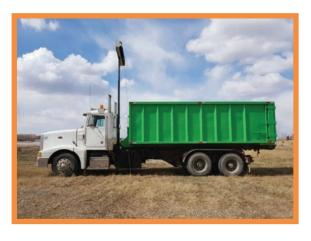
Single Leg Tower lifts 15' above the truck frame so the tarp can easily be pulled over the load
