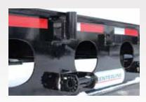
LOAD SECUREMENT This trailer is equipped with chain pockets opposite each crossemember and (10) load winches.
